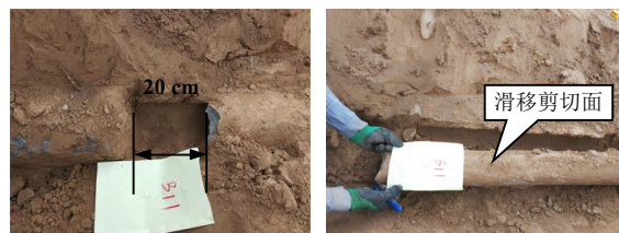
(a) 锚固长度为 3.5 m, BFRP 锚杆
