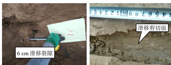
(c) 锚固长度为 3.5 m, 钢筋锚杆
